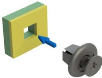
Light pressure to drive pin into fix
